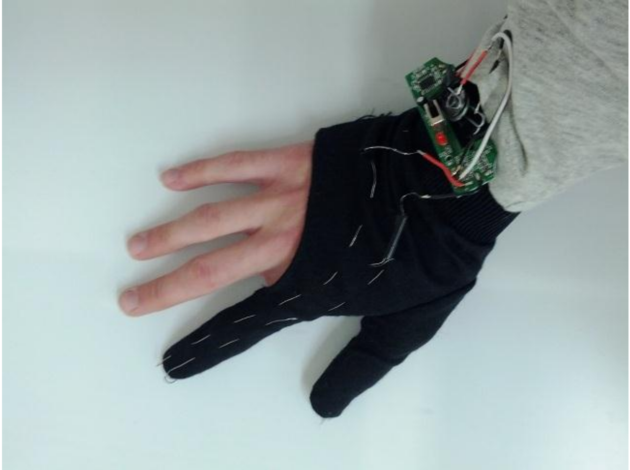
Figure 12 Final glove prototype with sewn circuitry
